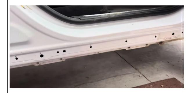
8. Moving to the front, with the front door open. Open up all the small round holes except the forward most one and the one that is obscured by the rear door.
