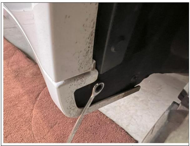
1. Remove 2x screws per corner holding in felt liner. 8 screws in total.
