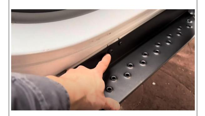
23. Fit all M6 black button head bolts and flat washers into the side of the slider into M6 nutserts.
