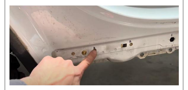
7. Starting from the rear, skip the first two holes and then mark the next 2. Open the holes to 9mm or imperial equivalent to suit M6 nutserts, skip the hex hole and the open the next hole.
